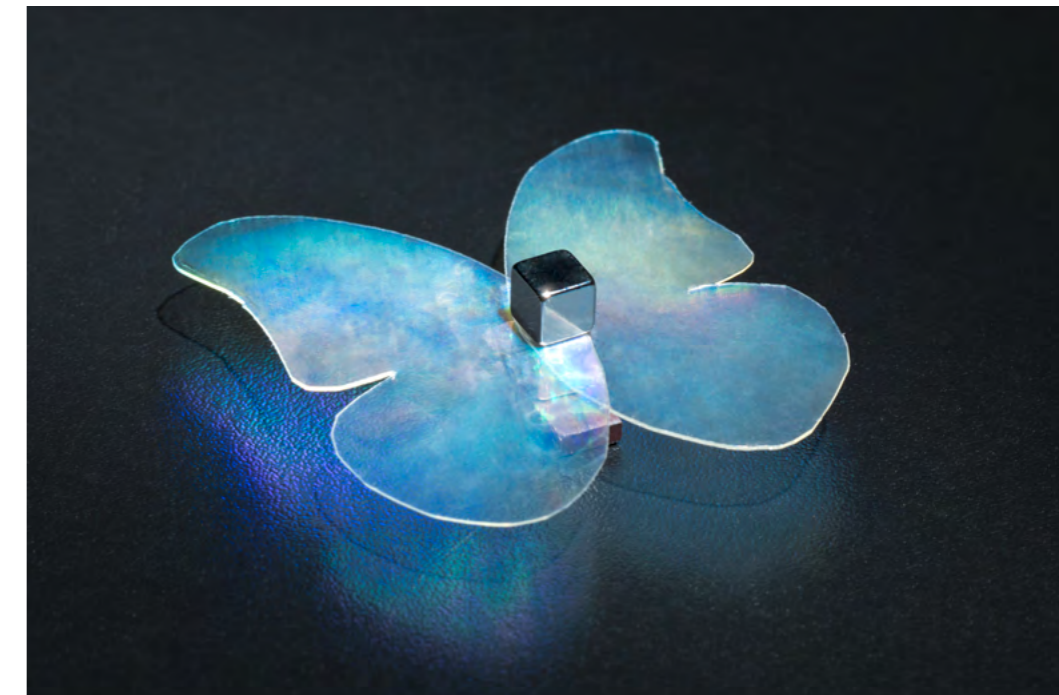
Nanostructures on the wing of Pachliopta aristolochiae can be transferred to solar cells and enhance their absorption rates by up to 200%.
