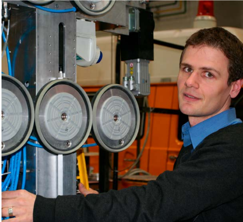
Professor Dr. Sascha Gentes presents the robot that autonomously decontaminates surfaces of nuclear facilities.
