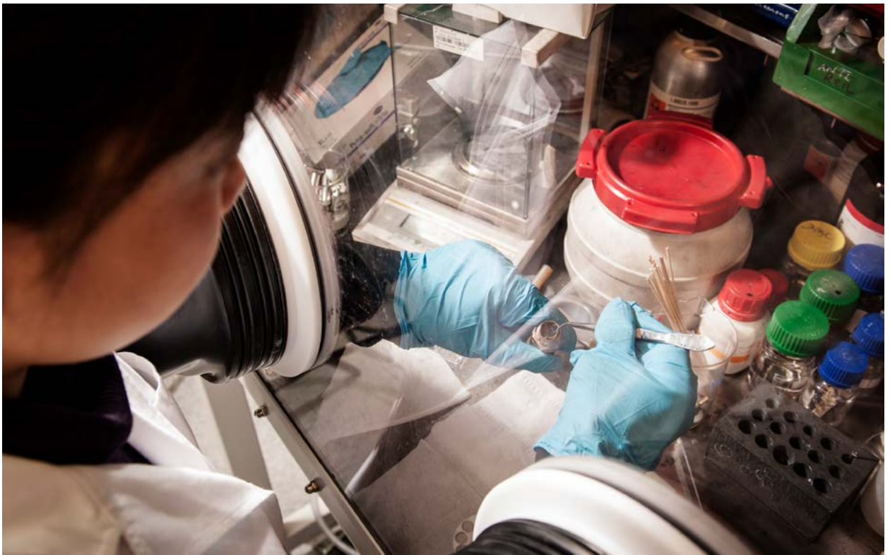
Test cells with the new cathode material are assembled in a glovebox.
