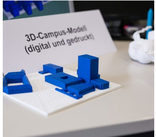
3D printers based on various printing technologies are used to make three-dimensional graphics tactile. (3D campus model (digital and printed))
