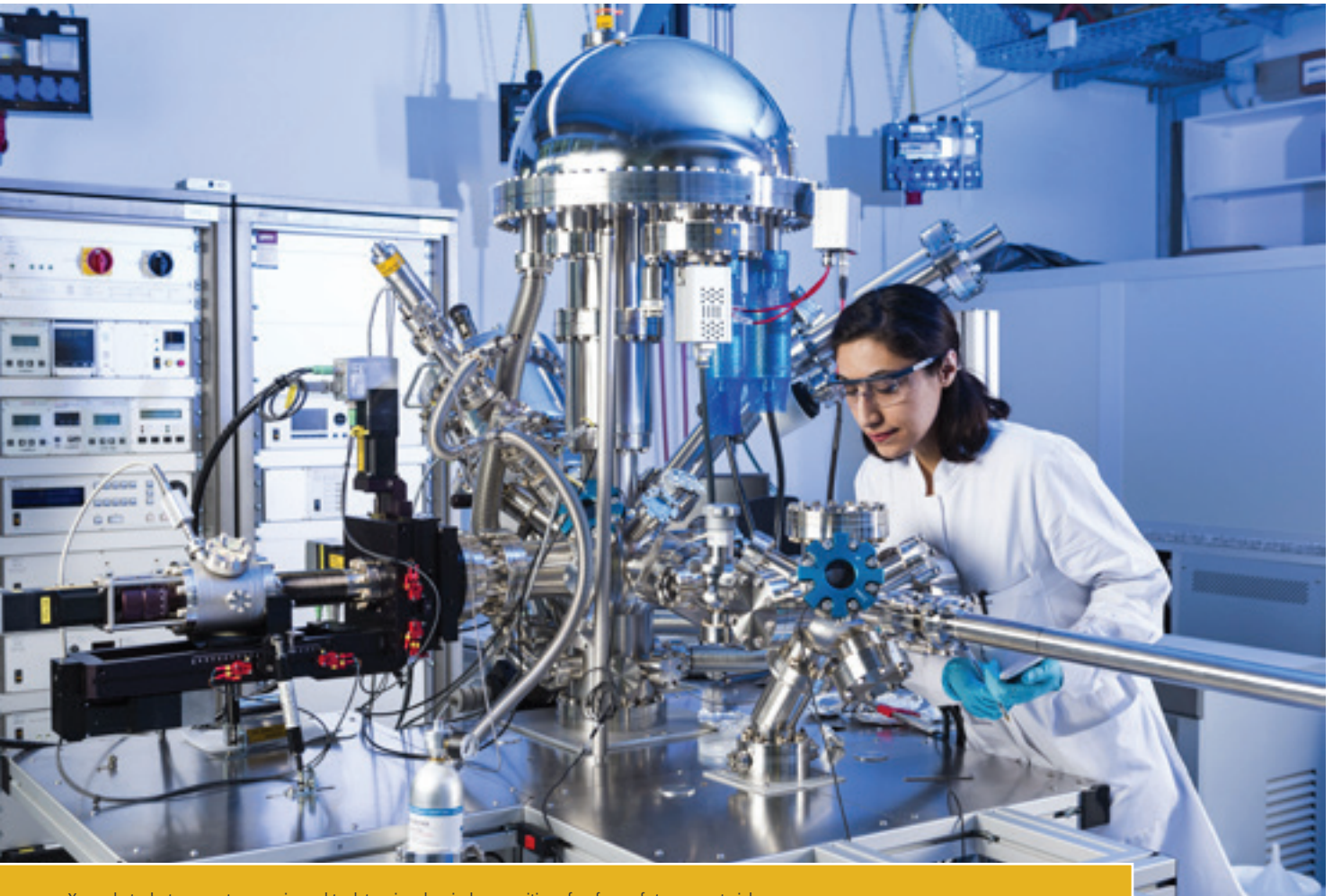
X-ray photoelectron spectroscopy is used to determine chemical composition of surfaces of storage materials.
