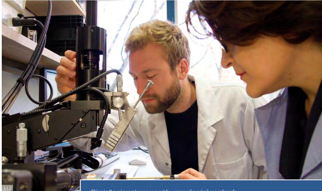
Chips in the micrometer range must be arranged precisely on a board.
